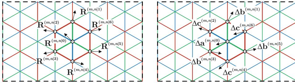
Figure 2: Resultant forces  $\mathbf{R}^{(m,n|i)}$  (left) and additional displacements  $\Delta \mathbf{u}^{(m,n|i)}$  (right) associated with the node  $i$  ( $i = 0, \dots, 6$ ) belonging to the cell  $\{m, n\}$  within the lattice drawn in its undeformed configuration.
