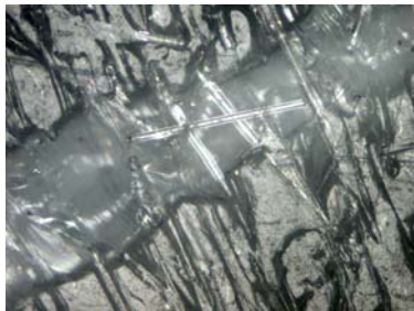
Figure 1: A bridged crack in short glass-fiber-reinforced polypropylene
