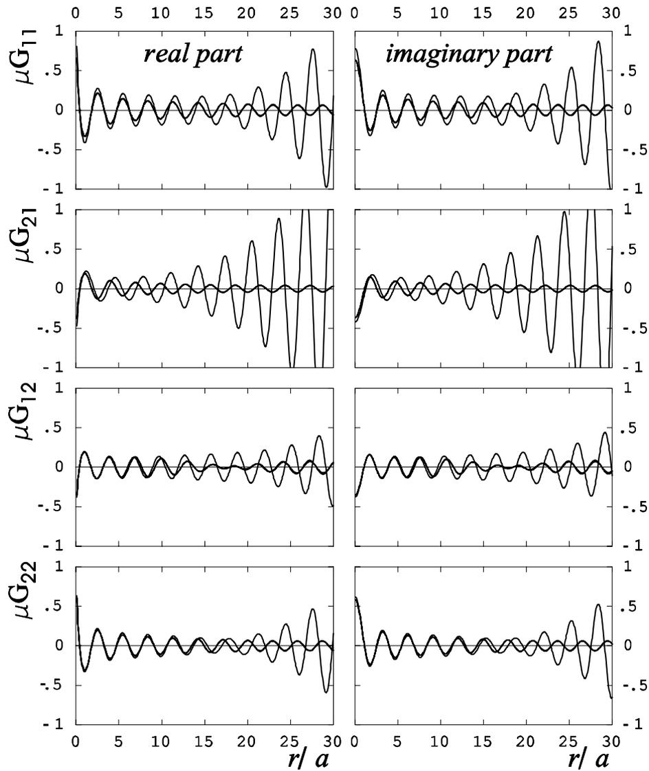
Fig. 4 Dimensionless Green's tensor components (real part left, imaginary part right in the figure) along a radial line inclined at  $-45^\circ$  with respect to the  $x_1$ -axis for Case 3 of Fig. 3 and  $\varpi = 1$ . Two values of the plastic modulus  $H/\mu = \{3.53, 1.5\}$  are considered, corresponding, respectively, to situations near and inside the flutter region. The blow-up of all components of the Green's tensor is evident in the flutter region,  $H/\mu = 1.5$ .
