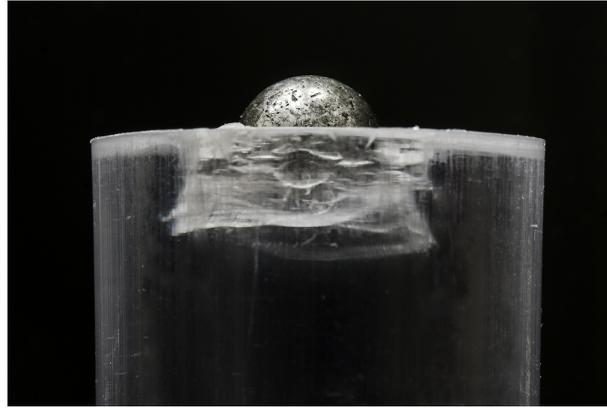
**Figure 1:** Conical fracture produced by a spherical indenter (14 mm diameter) at an indentation speed of  $8 \text{ mm s}^{-1}$  in a polycarbonate cylindrical specimen at  $0^\circ\text{C}$  (experiment performed by the authors at the Instabilities Lab. of the University of Trento).
