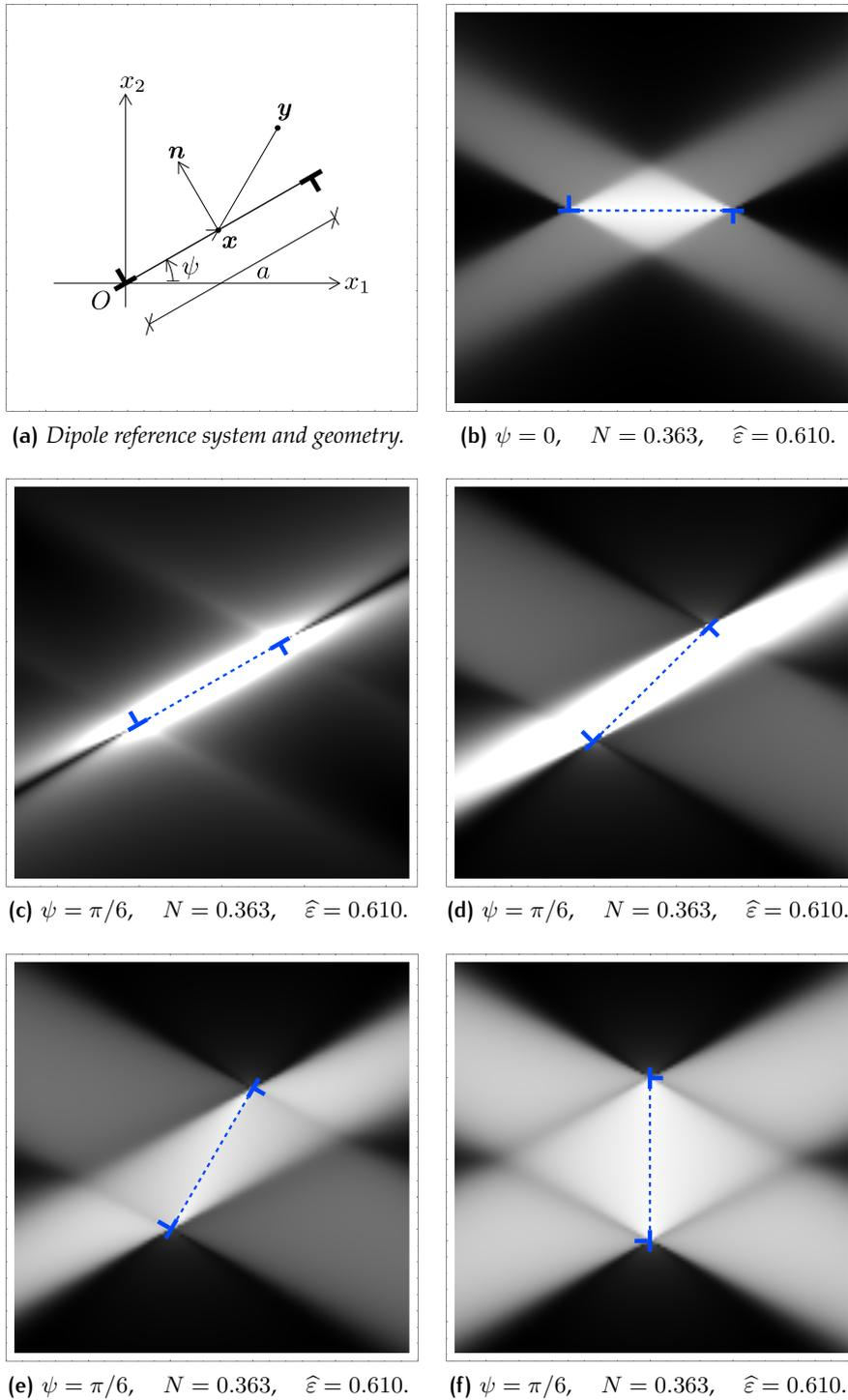
**Figure 6:** The (level sets of the modulus of incremental) displacement field produced by the emission of a straight edge dislocation dipole (of length  $a$  and inclination  $\psi$  with respect to the  $x_1$ -axis of orthotropy, see the geometrical setting in (a)) in a ( $J_2$ -deformation theory) plastic material, homogeneously deformed until near the elliptic boundary.
