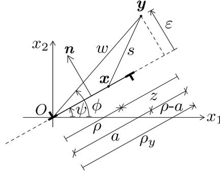
Figure 5: Infinite medium, including a straight *edge dislocation dipole* of finite length  $a$  and inclined at a constant angle  $\psi$  with respect to the  $x_1$ -axis.
