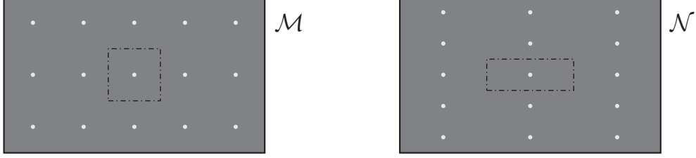
Figure 2: Two composites \mathcal{M} and \mathcal{N} containing a dilute suspension of isotropic circular inclusions in an isotropic matrix (with the same volume ratio f \ll 1 ). While standard homogenization leads to the same effective isotropic constitutive fourth-order tensor for both distributions, \mathbf{C}^{eq}(\mathcal{M}) = \mathbf{C}^{eq}(\mathcal{N}) , second-order homogenization leads to different effective nonlocal properties, \mathbf{A}^{eq}(\mathcal{M}) \neq \mathbf{A}^{eq}(\mathcal{N}) . In particular, while \mathbf{A}^{eq}(\mathcal{M}) is isotropic, \mathbf{A}^{eq}(\mathcal{N}) is orthotropic.
