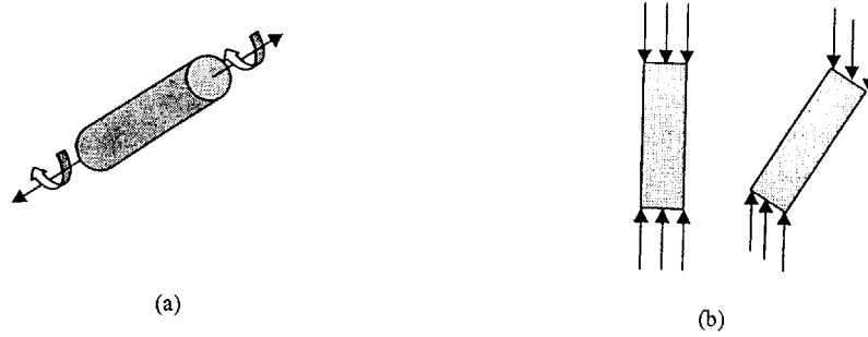
Fig. 1. a-neutral rotational equilibrium of a rod under tensile dead load; b-rotational instability of a rod under compressive dead load.
