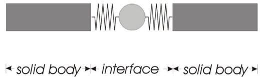
Figure 4. A simple model of structural interface with inertia
