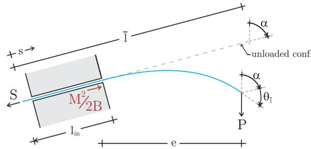
Figure 1: Structural scheme of the elastic system employed to disclose a Eshelby-like force. The elastic rod of total length  $\bar{l}$  is subject to a dead vertical load  $P$  on its right end, is constrained with a sliding sleeve inclined at an angle  $\alpha$  (with respect to the vertical) and has an axial dead force  $S$  applied at its left end. The presence of the Eshelby-like force  $M^2/(2B)$  influences the force  $S$  at equilibrium, which results different from  $P \cos \alpha$ .
