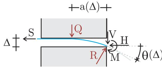
Figure 3: Deformed configuration of an elastic rod within an imperfect sliding sleeve made up of two smooth, rigid and frictionless planes placed at a distance  $\Delta$ . Applied and reaction forces provide in the limit  $\Delta \rightarrow 0$  the Eshelby-like force.
