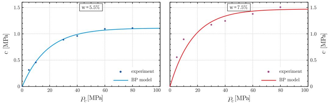
Figure 12: Cohesion parameter  $c$  as a function of the forming pressure  $p_c$ . Experimental data relative to aluminum silicate powder are compared to the model of increase of cohesion, eq. (4.6), proposed by Piccolroaz et al. (2006a) (solid line), evaluated with the parameters of Table 4, for water contents 5.5% (left) and 7.5% (right).
