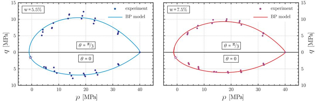
Figure 9: Meridian sections of the yield locus at Lode's angles  $\theta = \pi/3$  and  $\theta = 0$  for aluminum silicate green body formed under uniaxial strain at  $p_c^* = \sigma_1 = 40$  MPa, with water contents of 5.5% (left) and 7.5% (right). Yield points from triaxial tests (dots), evaluated through linear regression, and from equi-biaxial flexure tests (stars) are fitted with the BP yield surface (Bigoni and Piccolroaz, 2004), corresponding to the material parameters listed in Table 3.
