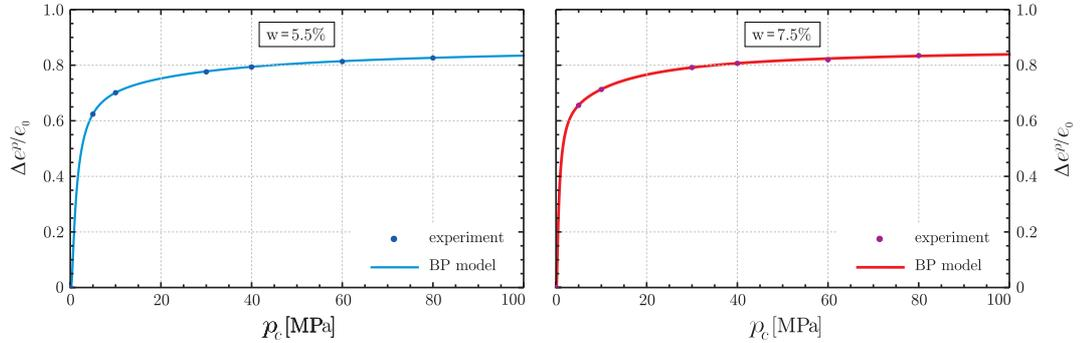
Figure 4: Plastic increment in the void ratio  $\Delta e^p$  as a function of the forming pressure  $p_c$ . Experimental data (dots) are compared with the Cooper and Eaton model, eq. (2.3), (solid line) for two water contents:  $w = 5.5\%$  (left) and  $w = 7.5\%$  (right). Note that there is a  $\approx 8\%$  (hardly visible) difference between the experimental values reported in the two graphs, due to the different water content.
