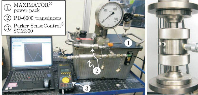
Figure 6: The experimental set-up for the high-pressure triaxial loading tests. Note the equipment to measure the lateral pressure (on the left) and the 45-D0554 Hoek cell inserted in the ZwickRoell Z250 electromechanical testing machine (on the right).
