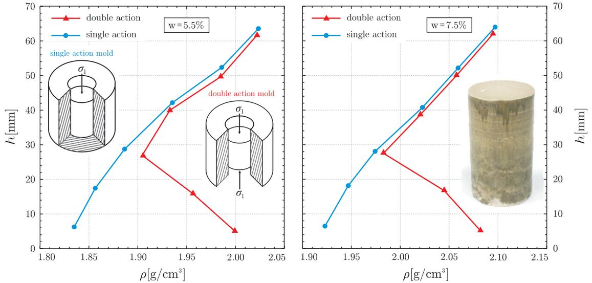
Figure 5: Mean (across the transversal area) density  $\rho$  distribution along the sample height  $h$  for water contents  $w = 5.5\%$  (left) and  $7.5\%$  (right). For each water content, the double pressure forming technique with a final pressure  $\sigma_1 = 40$  MPa is compared to the that obtained with the single action device. Note that the distributions of density are significantly more uniform in the former case than in the latter.
