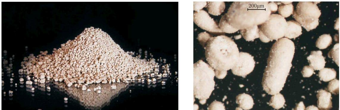
Figure 1: I14730 aluminum silicate spray dried powder in the loose state: bulk material (left) and micrograph at 31.5x (right, obtained with a Nikon stereoscopic microscope Nikon SMZ-800 equipped with Nikon Plan Apo 0.5x objective and a Nikon DS-Fi1 high-definition color camera head). The granules have an irregular surface and a mean diameter of 425  $\mu\text{m}$ .
