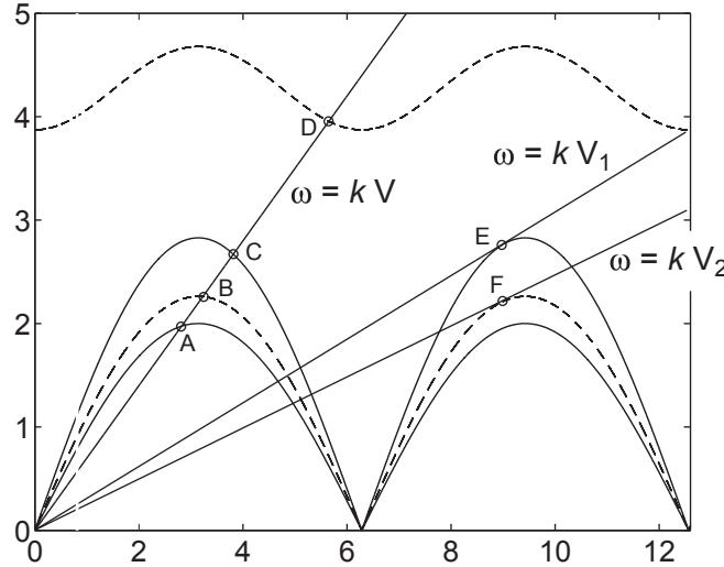
FIG. 4. Dispersion diagrams for  $s/c = 4$  as in Figure 3(a). Points E and F represent the resonant modes where the group velocity of the wave generated by the fault coincide with the speed  $V$  of the fault.
