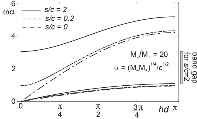
FIG. 6. Dispersion diagram for the intact structural interface shown in Figure 1.
