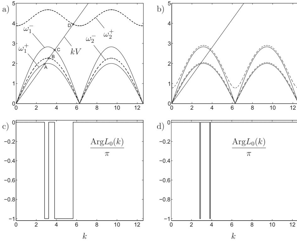
FIG. 3. Dispersion diagrams, determination of the zeroes of the functions  $Q_{\pm}(k)$ . Computations are reported for  $M_+/M_- = 4$ ,  $s/c = 4$ , and  $s/c = 0.2$  in (a) and (b), respectively. Evaluations of the functions  $\text{Arg } L_0(k)$  are reported in (c) and (d), corresponding to the two cases (a) and (b).
