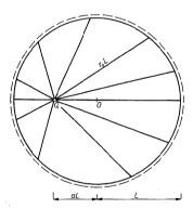
Fig. 7.10. Collapse mode for simply supported circular plate under eccentrically applied point load
