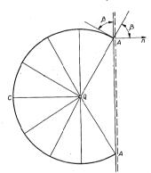
Fig. 7.17. Partial collapse of plate under point load in the vicinity of simply supported edge
