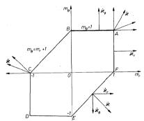
Fig. 4.3. Interaction curve for rotationally symmetric Tresca plates
