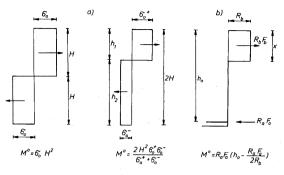
Fig. 2.7. Stress distributions at collapse for (a) homogeneous, (b) reinforced cross-sections
