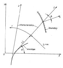
Fig. 8.2. Principal bending moment and curvature rate trajectories in the plate obeying maximum principal moment interaction curve
