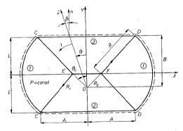
Fig. 8.9. Uniformly loaded simply supported plate
