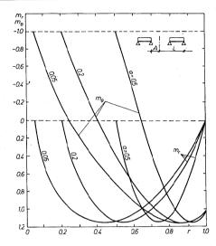
Fig. 4.15. Moment distribution in annular plate simply supported at both boundaries
