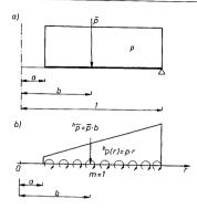
Fig. 4.9. Annular plate simply supported at outer edge: (a) support and load pattern of plate, (b) substitute beam pattern
