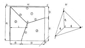
Fig. 7.6. Square plate with mixed boundary conditions: (a) yield line pattern,
