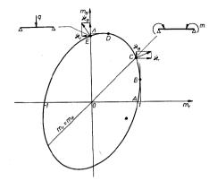
Fig. 6.5. Generalization of Huber-Mises ellipse to the orthotropic case
