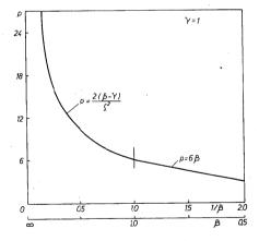
Fig. 6.14. Collapse load for uniformly loaded simply supported orthotropic plate obeying interaction curve shown in Fig. 6.11a
