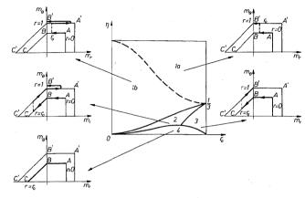
Fig. 6.4. The ranges of validity of the solutions for a nonhomogeneous circular plate with a weaker central part
