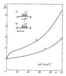
Fig. 4.5. Total collapse load for step-wise loaded circular plate: (a) simply supported,
