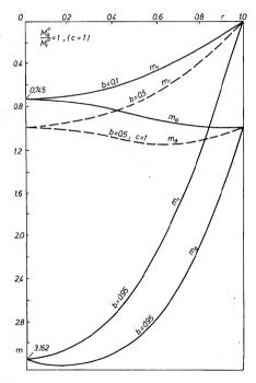
Fig. 6.7. Distribution of moments in circular simply supported orthotropic plate for parameters c=1 and b=0.1 and 0.95
