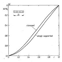
Fig. 4.12b. Characteristic diagrams for Huber-Mises circular plates - deflection rates
