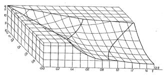
Fig. 7.21. Level curves of a constant load carrying-capacity for rectangular simply supported plate under point load
