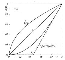
Fig. 6.17. Deflection rates for simply supported orthotropic circular plate obeying interaction curve shown in Fig. 6.11a
