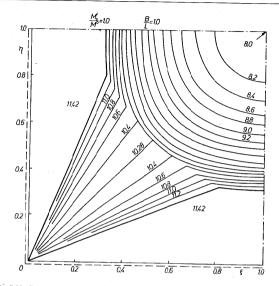
Fig. 7.20. Contour map of load-carrying capacity for a square plate under point load
