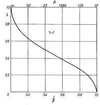
Fig. 6.12. Hinge circle radius  $r_A$  against the ratio of orthotropy  $\beta$
