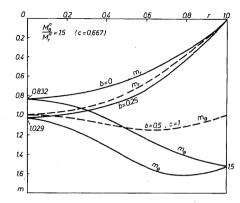
Fig. 6.8. Distribution of moments in circular simply supported orthotropic plate for parameters c = 0.667 and b = 0 and 0.25
