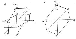
Fig. 6.11. Stress profile for orthotropic simply supported circular plate obeying: (a) asymmetrical, (b) symmetrical piece-wise interaction curve
