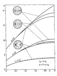
Fig. 8.8. Comparison of the exact and the yield line solutions for simply supported circular plate under two point loads
