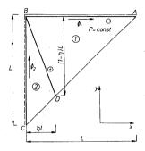
Fig. 7.7. Yield line pattern in uniformly loaded corner plate with mixed boundary conditions
