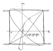
Fig. 3.4. Interaction surface for reinforced slabs
