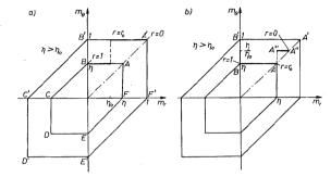
Fig. 6.2. Stress profiles for nonhomogeneous simply supported circular plate with a stronger central part: (a) total yielding, (b) partial yielding
