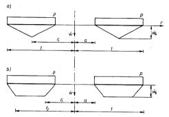
Fig. 4.7. Two collapse modes for Johansen annular plate
