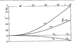
Fig. 6.16. Moment distribution in simply supported orthotropic circular plate obeying interaction curve shown in Fig. 6.11a
