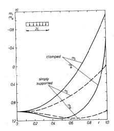
Fig. 4.12a. Characteristic diagrams for Huber-Mises circular plates — moment distribution
