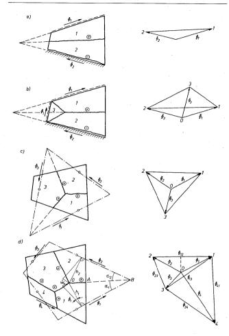
Fig. 7.2. Yield line patterns and rotation rate diagrams for four examples of plates
