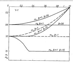
Fig. 6.13. Moment distribution in simply supported orthotropic circular plate obeying interaction curve shown in Fig. 6.11a
