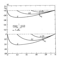
Fig. 4.14. Moment distribution in Huber-Mises plates simply supported (a) at outer edge, (b) at inner edge
