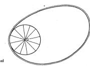
Fig. 7.12. Collapse mode of a point loaded clamped plate
