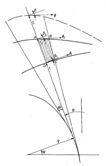
Fig. 7.14. Infinitesimal strip bounded by two arbitrarily curved hinges
