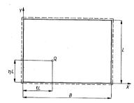
Fig. 7.19. Simply supported rectangular plate under point load
