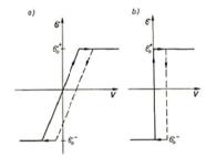
Fig. 2.1. (a) Elastic-perfectly plastic, (b) rigid-perfectly plastic models of materials
