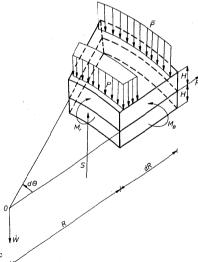
Fig. 4.1. Rotationally symmetric plate element in polar coordinates
