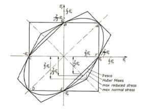
Fig. 2.2. Comparison of Huber-Mises, Tresca, maximum reduced stress and maximum normal stress yield criteria
