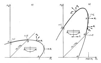
Fig. 6.6. Two variants of collapse for circular simply supported orthotropic plate obeying nonlinear interaction curve
