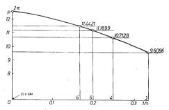
o - numerical results n - number of polygon sides moments, shear forces, deflection rates as for square plate (plate 49) PLATE 51, [48]
