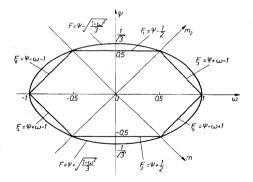
Fig. 3.5. Huber-Mises and Tresca interaction curves in the plane of invariants  $\omega$ ,  $\psi$
