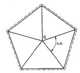
Fig. 7.8. Yield line pattern in polygonal simply supported plate under point load
