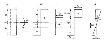
Fig. 2.8. Bending and stretching of beam: (a) generalized stresses, (b) stress distribution at collapse, (c) generalized strain rates
