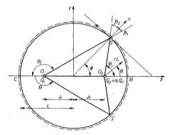
Fig. 8.7. Simply supported circular plate under two point loads
