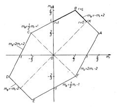
Fig. 4.2. Maximum reduced stress interaction curve for rotationally symmetric plates
