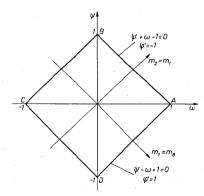
Fig. 8.1. Maximum principal moment interaction curve in the plane of the moment invariants
