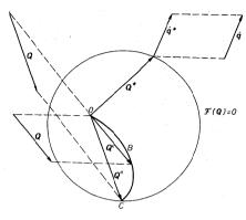
Fig. 2.10. Admissible states: statically admissible stress field Q<sup>0</sup> and kinematically admissible strain field o'\* with associated stress field Q\*
