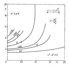
Fig. 6.10. Collapse load for uniformly loaded circular simply supported orthotropic plate
