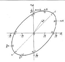
Fig. 4.10. Huber-Mises interaction ellipse for rotationally symmetric plates
