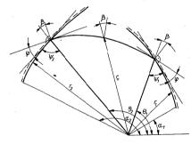
Fig. 7.13. Polar yield line fan bounded by a negative yield line and contained within two simply supported edges
