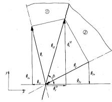
Fig. 7.3. Rotation vector of two adjacent plane portions about the yield line and its components
