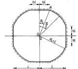
Fig. 8.5. Simply supported square plate with rounded corners
