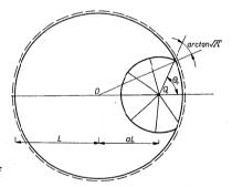
Fig. 7.18. Partial collapse of circular simply supported plate
