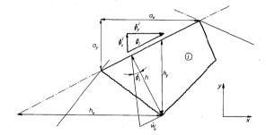
Fig. 7.4. Rotation vector of the i-th plane portion about the supported edge and its components
