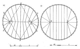
Fig. 7.15. Deflected surface for simply supported circular plate loaded by two equal point loads: (a) consisting of conical elements, (b) consisting of conical and cylindrical elements
