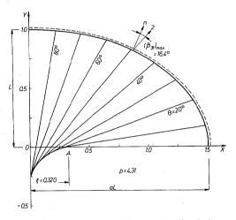
Fig. 8.11. Elliptic simply supported plate under uniform load
