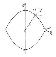
Fig. 2.9. Interaction curve for bending and stretching of beam with rectangular cross-section
