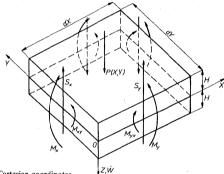
Fig. 3.1. Plate element in Cartesian coordinates
