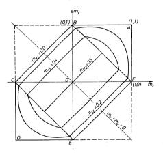
Fig. 3.3. Interaction surface for Tresca plates
