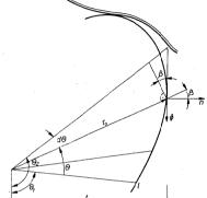
Fig. 7.11. Yield line fan bounded by a negative yield line  $r_0 = r_0(\theta)$
