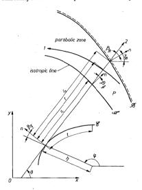
Fig. 8.10. Partially loaded fragment of simply supported plate
