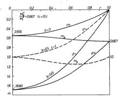
Fig. 6.9. Distribution of moments in circular simply supported orthotropic plate for parameters c=1 and b=0 and 1.45
