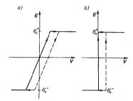
Fig. 2.1. (a) Elastic-perfectly plastic, (b) rigid-perfectly plastic models of materials
