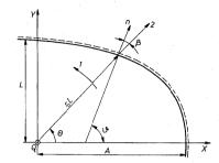
Fig. 8.3. A quarter of simply supported elliptic plate loaded at its centre
