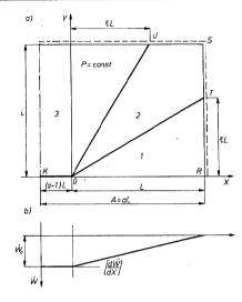
Fig. 5.1. Simply supported and uniformly loaded rectangular plate: (a) yield line pattern, (b) deflection rate
