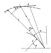
Fig. 7.9. Yield line fan developed from an envelope
