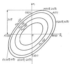
Fig. 3.2. Interaction surface for Huber-Mises plates
